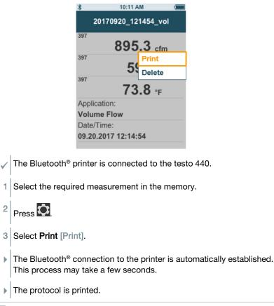
During printing, the testo 440 interrupts the Bluetooth<sup>®</sup> connection to the connected probe. The connection is automatically restored after printing has finished.
