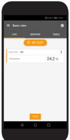
The cost-free testo Smart App turns your smartphone/tablet into the display for the testo 915i. The operation of the Smart Probe and the display of the measurement values take place wirelessly by Bluetooth<sup>®</sup> on your smartphone – independently of the measurement location. In addition, you can use the App to create measurement reports, add photos and comments to these and conveniently send them by e-mail.
